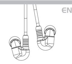
Insert the earphones into the ear canal with the cable facing up and slightly twist it backward until the sleeves feel like sealing the ea
