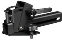
swiveling fastening solution for horizontal and vertical alignment, for flown / ground stacked / mounted applications, incl. accessories (2 x star knob screws M10 x 18 mm, 1 x handle screw M8 x 55 mm), max. load 50 kg
