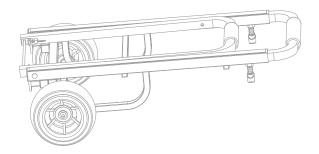
To unlock and expand the frame step carefully on the steel cable.
