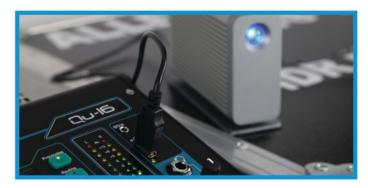
A selectable stereo pair can be recorded alongside the 16 Mono channels, and multitrack audio can be played back to the 16 Mono channels plus ST1.
