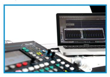
The returns from the Mac can be assigned to the 16 Mono channels plus stereos.
