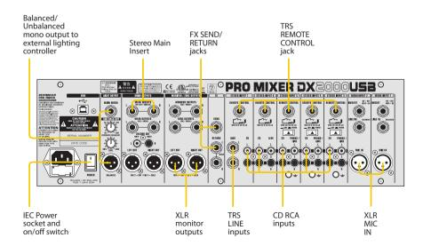
music's strongest pulses with a lighting system, provided your lighting system has "sound-to-light" capability (e.g. BEHRINGER LC2412 Lighting Console). The Main Output section offers balanced 1/4" TRS and XLR stereo outputs, as well as 1/4" TRS Main Insert jacks for connecting to outboard EQ and dynamics processors, such as limiters and
