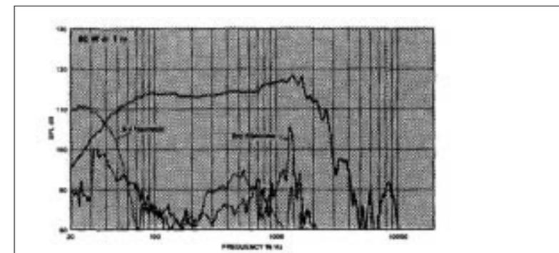
Distortion levels raised 20 dB, measured at 60 watts, 1 meter.
