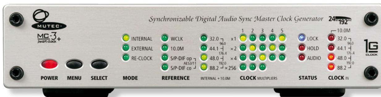
exist for externally supplied clock references (WCLK or 10 MHz). The capture range covers 25 to 200 kHz, 10 MHz and both Super Clock frequencies. Finally, one can also use the MC-3+ as a 'format converter' for digital audio and clock signals. Among the possibilities are AES3/AES11/S/P-DIF, WCLK/AES11 and 10M/WCLK/AES11, each in any combination and direction.
