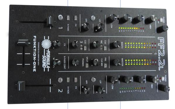
Each channel has 2 inputs, 12 LED meter, 4 band full kill EQ, FX loop and adjustable high and low pass filters.
