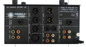
The FX switch on each channel sends that channel to the 1/4" send jack and routes the FX return 1/4" jack returns to that channel. ie it acts like an insert for whichever channel selects FX.
