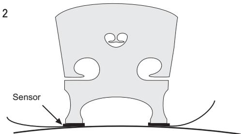
2. If pickup is too loose, shim with included shim material (see fig 3). If pickup is too high, file the bridge slot slightly.
