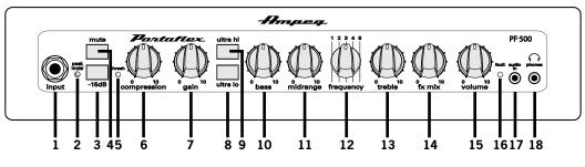
**18. PHONES:** Use this 1/8" TRS stereo output to connect your headphones. The output here is a mix of the line-level signals reaching the amplifier, and any incoming audio from the audio in jack [17].
