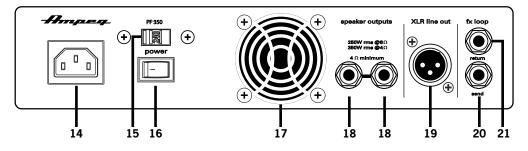
**20. FX SEND JACK:** Use this 1/4" TS unbalanced output to send a line-level output to an external effects processor (for example). The output here is affected by all controls except the volume.
