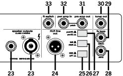
**23. SPEAKER OUTPUTS:** These individual Speakon / 1/4" TS output jacks supply speaker-level power to the speaker cabinet. The rated power output is 300 watts rms into 8 ohms or 500 watts rms into 4 ohms.
