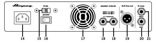
IEC POWER INPUT CONNECTOR: This is where you connect the supplied AC power cord.
