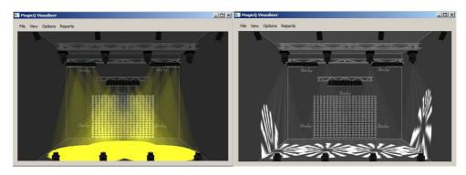
MagicVis is available in two versions. MagicQ has the visualiser combined into it for use on PCs and Macs. In addition a stand alone MagicVis application can be run on a laptop connected via network to a MagicQ console.
