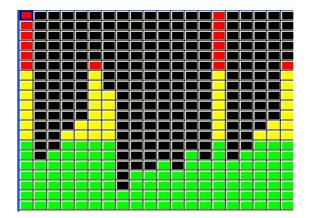
Ramp Horiz and Ramp Vert – these perform a ramp across the entire grid in the horizontal or vertical directions. FX P1 parameter controls the speed, FX P2 controls the crossfade and FX P3 controls the width.
