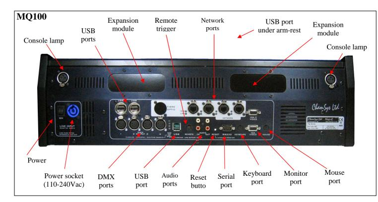
MagicQ MQ100 Expert consoles have a similar rear panel but with only one network port and two (non locking) USB ports. MQ100 Expert consoles do not have VGA ports for additional monitors.
