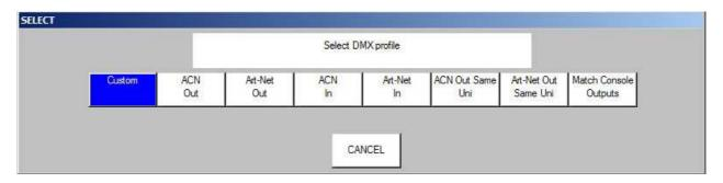
The profiles act as a starting point – once a starting profile has been chosen, the detailed configuration can all be set individually for each port by changing to the VIEW PORTS view.
