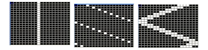
Vert random, Horiz random – enable random movement of elements across the grid. Modify the mode to change thickness of the elements and offset to change the frequency. With this FX it is possible to generate snow and rain type FX.
