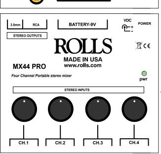
OUTPUTS: 1/4" and 1/8" (3.5 mm)Tip-Ring-Sleeve jack for connection to a mixer input, amplifier or other input device.
