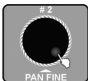
4. Turn jog wheel # 2 to select the position (Step) to be changed. The display shows the 'Step' number and the respective scene is displayed.
