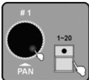
3. ➤ Press the number button [1 – 20] of the Cue that you want to edit. The LED of the [CHASE] button as well as the button LEDs of the Chases used in the Cue light up while the Cue runs. The LEDs of those buttons where Chases are stored, that are not used in the Cue, are flashing. Turn jog wheel # 1 to access the Chases stored on other memory pages.
