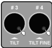
3. Rotate jog wheel # 3 or # 4 to adjust the value for speed (0-255) or dimmer (0-255) of a DMX strobe.
