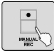
4. ➤ Then press the *[MANUAL/REC]* button to initiate the saving. The LEDs of the buttons CUE, OVERRIDE, CENTER, FIXTURE GROUP, PRESET, CHASE, BANK and BLACK OUT are flashing.
