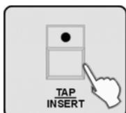
**5.** Press the [TAP/INSERT] button to insert a scene after the current position.
