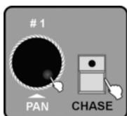
1. ➤ Press the [CHASE] button. Turn jog wheel # 1 to select the memory page on which the desired Chase is stored. Now the LEDs of those number buttons light up where Chases have already been stored.
