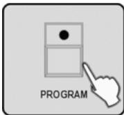
Enter the programming mode by holding down the *[PROGRAM]* button for 2 seconds. The LED of the *[PROGRAM]* button flashes when the programming mode is activated.
