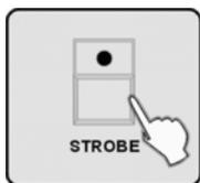
5. ➤ Press the *[STROBE]* button to let the Invader control the DMX strobe according to the adjusted values.
