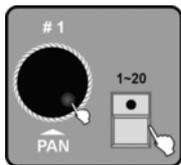
**5.** Rotate jog wheel # 1 to select the bank that contains the scene that you want to insert. Press the number button [1 – 20] of the scene to be added to the chase in the current step.
