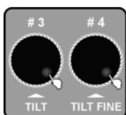
3. ➤ Turn jog wheel # 4 to select a profile from the STAIRVILLE profile collection. Turn jog wheel # 3 to select a profile from the profile collection of another manufacturer ('other profiles'). The respectively selected profile name appears at the bottom left in the display.
