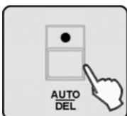
3. ➤ Hold down the [AUTO/DEL] button while pressing the number button [1 – 20] where the Cue is stored that you want to delete. All LEDs flash three times and thus indicate the successful deletion of a Cue.
