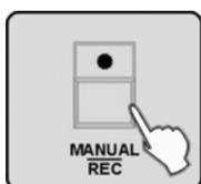
**9.** Press the [MANUAL/REC] button. All LEDs flash three times and thus indicate the successful insertion of a scene.
