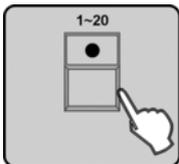
4. ➤ Press the number button [1 – 20] to deselect currently used Chases or to add new ones. For timing control, turn the jog wheels # 3 (Fade Time) & # 4 (Wait Time).
