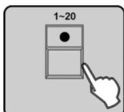
**7.** Press the number button *[1 – 20]* to select the number for the Override to be saved. All LEDs flash three times and thus indicate the successful programming of an Override.
