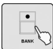
1. ➤ Press the [BANK] button. Now the 'MANUAL' LED should light up. Otherwise press the [MANUAL/REC] button to call up the manual mode.
