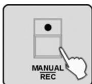
7. ➤ Press the [MANUAL/REC] button - now the LEDs of the buttons CUE, OVERRIDE, CENTER, FIXTURE GROUP, PRESET, CHASE, BANK and BLACK OUT are flashing.
