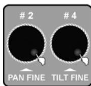
5. If desired, turn jog wheels # 2 and # 4 to change to the name of the device. Rotate jog wheel # 2 to change the cursor position. Turn Jog wheel # 4 to change the character. You can choose from 26 letters and 10 numbers as well as the special character '—'. The max. length of the device name is 16 characters.
