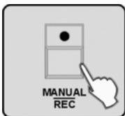
5. ➤ Press the [MANUAL/REC] button. All LEDs flash three times and thus indicate the successful editing of a Cue. The Cue run is stopped then.
