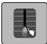
**4.** Use the channel faders or the jog wheels # 1–# 4 to adjust the desired effect.
