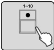
7. ➤ Press one of the number buttons [1 – 10] to save the colour settings as a COLOR preset, or press one of the number buttons [11 – 20] to save the gobo settings as a GOBO preset.. All LEDs flash three times and thus indicate the successful saving of a preset. All set DMX values that are not related to colour and gobo are not saved.
