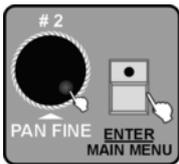
3. ➤ Rotate jog wheel # 2 to toggle between 'power on password', default setting) and 'memory protect password'. Press the [ENTER / MAIN MENU] button to activate the selected function.
