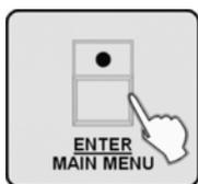
4. ➤ Press the [ENTER / MAIN MENU] button to confirm, all LEDs blink three times. Then, the device will quit this submenu.
