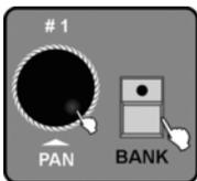
7. ➤ Press the [BANK] button and turn Jog wheel # 1 to select the memory bank, in which the scene is to be stored.
