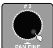
**4.** Turn jog wheel # 2 to select the scene to be deleted with the help of the 'Step' display.
