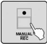
5. ➤ Press the [MANUAL/REC] button. All LEDs flash three times and thus indicate the successful saving of a Cue.
