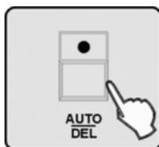
4. ➤ Hold down the *[AUTO/DEL]* button while pressing the number button of the scene to be deleted. All LEDs will flash three times briefly to confirm the procedure.
