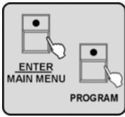
4. Press the *[ENTER/MAIN MENU]* button to save the settings. Press the *[PROGRAM]* button to leave the menu.
