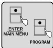
3. ➤ Press the *[ENTER/MAIN MENU]* button to save the settings. Press the *[PROGRAM]* button to leave the menu.
