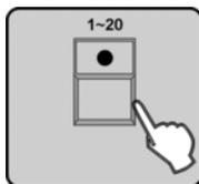
6. ➤ Press a number button *[1 – 20]* to copy the scene to the desired position. All LEDs will flash three times briefly, thus indicating that this step has been completed successfully. The display then shows the number of the bank along with the number of the copied scene.
