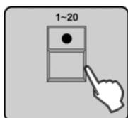
6. ▶ Now the LEDs of those number buttons light up where scenes have already been assigned to. Press the desired number button *[1 – 20]* where the scene is to be stored. Already occupied memory slots are overwritten without prompting. All LEDs will flash three times briefly to indicate the successful saving. Also, the display confirms the saving with *'Store a scene succeed'*. Underneath appears the indication of the bank number and the number of the newly programmed scene.
