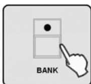
1. ➤ Press the [BANK] button and turn jog wheel # 1 to select the desired bank 1 – 60.
