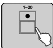
2. ➤ Press the number button [1 – 20] to select the desired chase. You can also select multiple chases. Their numbers will be indicated in the display. The number of the currently active Chase is flashing then. To activate the respectively next Chase, press the number button [1 – 20] of the currently active Chase in order to deactivate it.
