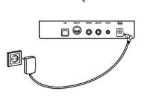
Connect the cable from the power supply outlet to the input socket [12V] on the rear panel of the piano. Plug the plug of the power cord into a properly wired and earthed mains wall outlet.
