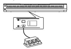
Use the connection socket on the bottom of the digital piano to connect the triplepedal (Sustain, Sostenuto and Soft) of the optional Thomann original stand (item no. 352262).
