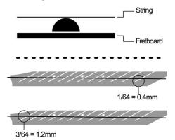
At the first fret, the distance between string and fretboard should be approx. 0.4 mm, at the twelfth fret approx. 1.2 mm. If necessary, check the connections and positioning of the components.
