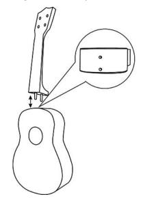
The neck is fastened with a tongue and groove connection to the body. First, check whether the connection between neck and body fits correctly. Wood slightly changes its shape over time. If the neck sits too tight in the groove on the body, a slight adjustment with a sharp wood chisel or sandpaper may be needed.
