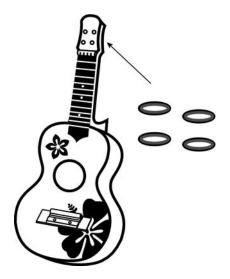
Press the four fixing rings for the machine heads from the front into the respective holes of the headstock.
