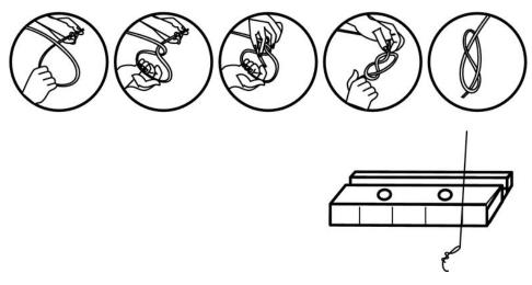
The package includes a set of strings for the Hawaiian tuning (G - C - E - A). Tie a knot at one end of the strings (simple knot for the two thicker strings, double knot for the two thinner strings) and insert the strings into the grooves of the bridge as shown in the figure:
