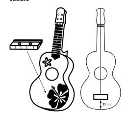
The bridge is to be glued in the middle of the body surface and fixed with the two long screws. First mark the correct position of the bridge on the body surface. Note the spacing dimensions shown in the figure.
