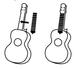
The fretboard is glued to the neck. Apply wood glue on both surfaces. Position the fretboard on the neck and align it so that at the base of the headstock a 5 mm clear space remains for mounting the nut. To dry the adhesive joint, fix the fretboard with rubber rings on the neck.
