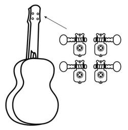
Insert the four machine heads from the rear side of the headstock into the holes provided.
