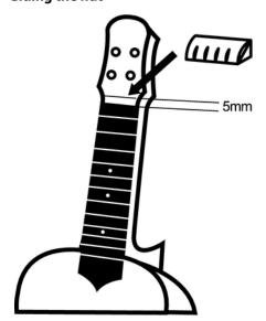
The nut is to be glued above the fretboard on the neck (needed clearance between fretboard and headstock 5 mm, see previous section). Apply wood glue on both surfaces. Put the nut on the neck and fix it to dry the adhesive joint with rubber rings on the neck.
