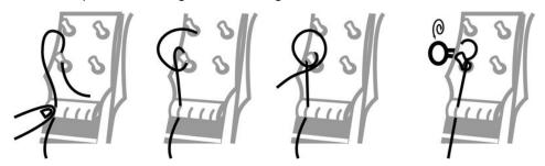
Thread the loose ends of the four strings into the holes of the designated machine heads. Make sure to attach each of the four strings with two to three turns securely to the tuning pins (see figure). First, slightly pre-tighten all strings and check the action as described in the following section.
