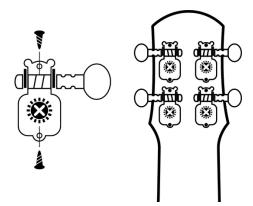
Fasten the four machine heads with two short screws each.
