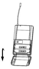
The battery compartment of the UHF pocket transmitter is located on the back of the device.
