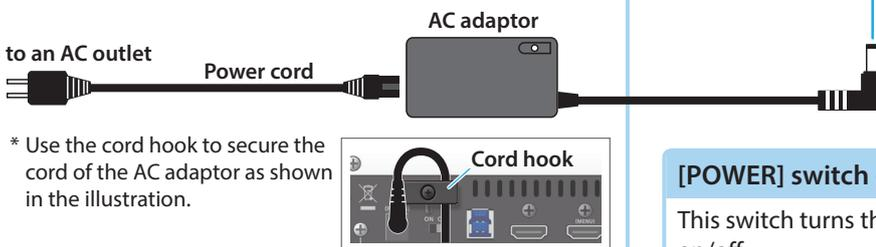
\* Use the cord hook to secure the cord of the AC adaptor as shown in the illustration.
