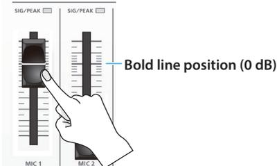
2. Move the [MAIN] knob to a position near the indicator (0 dB).
