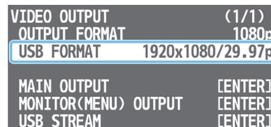
2. Turn the [VALUE] knob to select the output format, and press to confirm.
