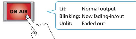
The main output video fades-out to a black screen. When fade-out is complete, the [ON AIR] button goes dark.
