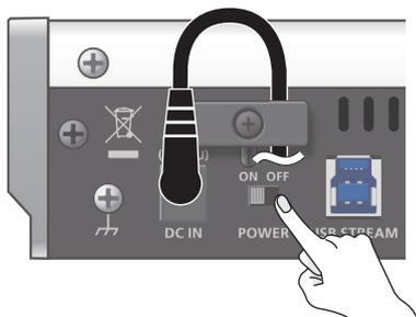
3. Turn on the power in the order of source devices → output devices.
