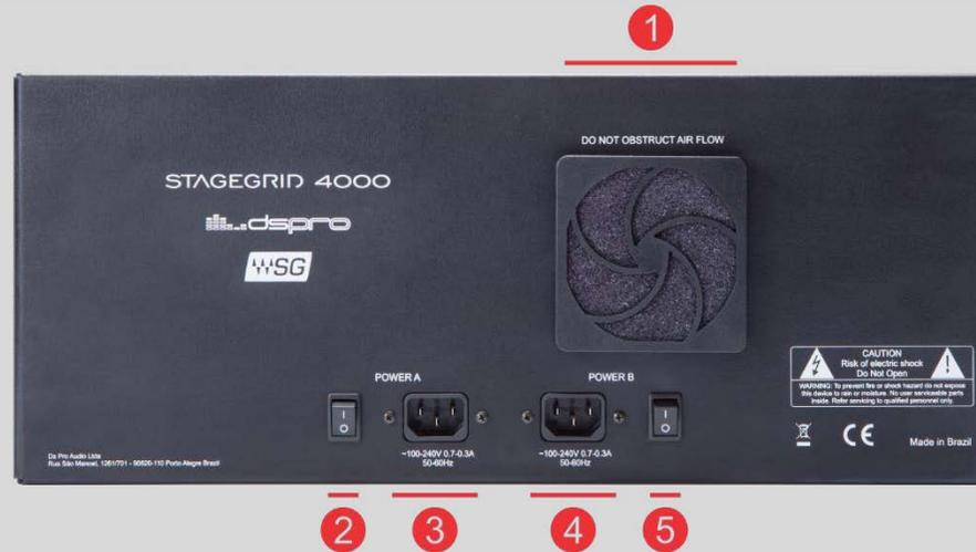
1. Device fan. Air flows from the back to front and sides.
