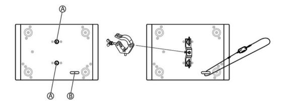
The threads on the bottom side of the housing (A) allow the secure attachment of the included mounting bracket. There, you can fasten adapters such as half couplers, trigger clamps, chooks etc. Safety cables are being threaded through the eyelet (B) on the bottom side of the housing.
