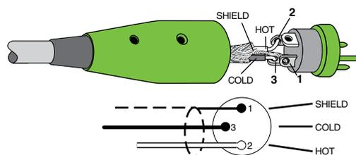
In addition to accepting balanced mic or line-level signals using an XLR connector, both channels may also accept 1/4" line-level signals driven by balanced or unbalanced sources.
