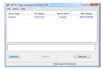
NMU (Node Management Utility) is a free Windows and Mac application that is used to manage compatible ENTTEC DMX over Ethernet nodes. NMU will not directly allow you to configure the Pixelator itself, but it can help you find your unit's IP address and then open a browser window to access Pixelator. Follow these steps:
