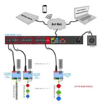
With the default profile, each Pixel Link port is mapped to its respective Art-Net Universe, allowing you to directly plug-in your Pixelator without the need for configuration.
