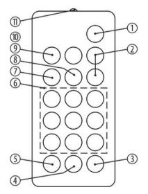
To use the remote control, point its infrared diode at the infrared sensor on the unit and press the desired buttons. The maximum operating distance is about 9 m. The device will only respond to the remote control signals if it is not controlled via DMX.
