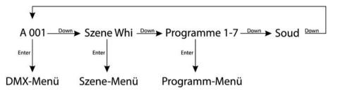
Press [DOWN] while 'A001' is flashing in the display to call up the preprogrammed scene. Press repeatedly [DOWN] to call one of the 7 programmes. If necessary, press repeatedly [DOWN] to set the device to sound-to-light mode.
