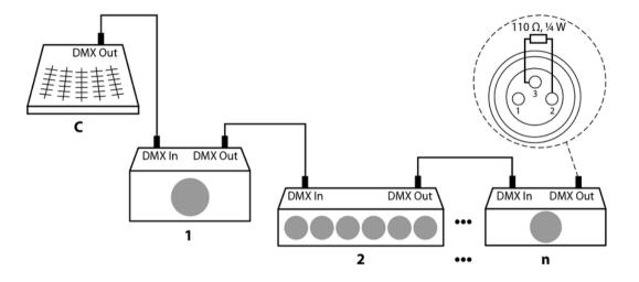
Connections in 'Master / Slave' mode When you configure a group of devices in 'Master / Slave' mode, the first device controls the others and allows an automatic, music-controlled and synchronized show. This feature is especially useful to start a show without much programming. Connect the DMX output of the master unit to the DMX input of the first slave unit. Then connect the DMX output of the first slave unit to the DMX input of the second slave unit and so on (maximum 30 slaves).
