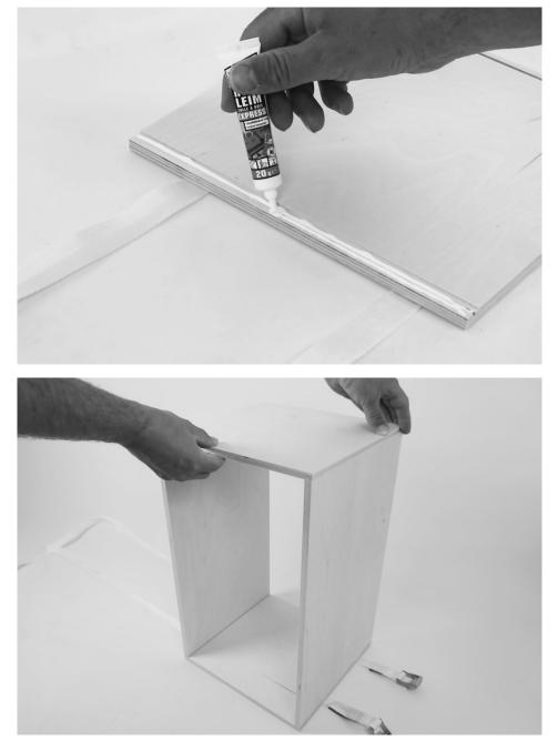
After you have glued the two side panels to the floor panel check them for flushness and glue the top plate in the same way.
