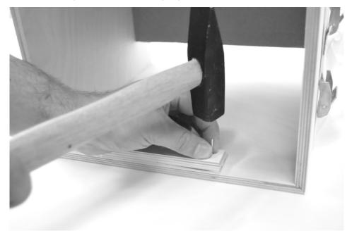
Fix the snare strip with two nails in the pre-punched holes.
