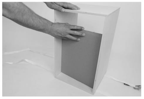
Slide the supplied cardboard angle template centrally into the body to create a straight angle.
