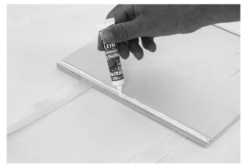
Apply the express glue carefully in the entire groove and the adjoining surface of the base plate. Glue residues can be removed with a damp cloth.
