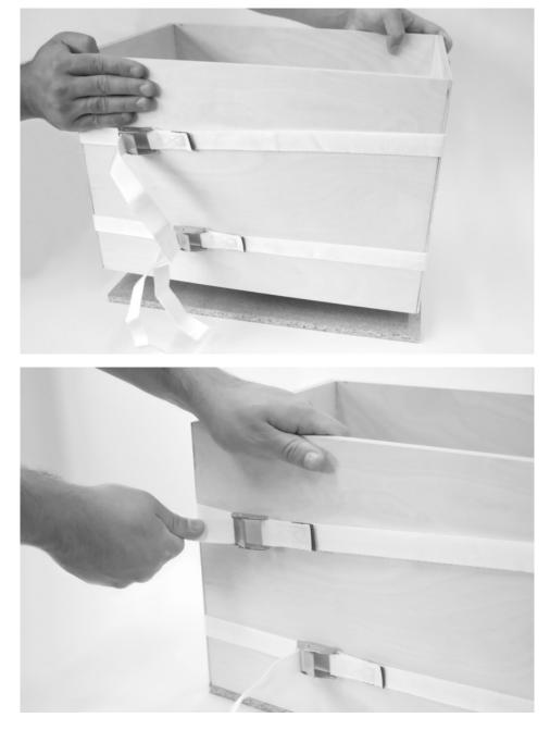
Place the cajon horizontally on the pressure plate and check the connections for flushness. Readjust them, if necessary, and tighten the tension straps.
