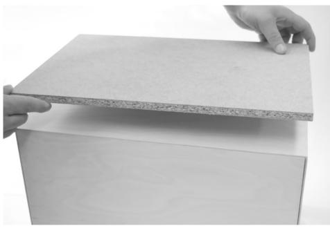
Put the pressure plate on the striking surface, check the edges for flushness and press the pressure plate briefly.
