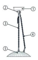
A suitable safety bolt is part of the delivery and is used to attach a safety chain, which must secure the attached mirror ball against falling.
