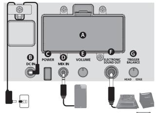
The ELCajon can operate on batteries or on the included AC adaptor. If you are using batteries, insert six AA batteries, making sure that the batteries are oriented correctly.
