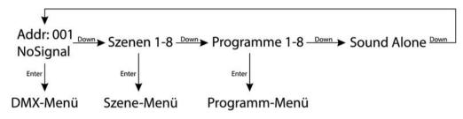
Press repeatedly [DOWN] while 'A001' is flashing in the display to call up one of 8 preprogrammed scenes, one of 8 programmes or to set the device to sound-controlled mode.
