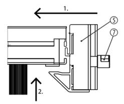
Slide the mounting clamps (5) for the railings (4) into the profiles of the respective stage platforms. As shown in the following figure, the guiding stub of the mounting bracket in the profile must be aligned upwards.
