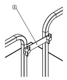
If more railings are required, attach them to the stage platforms first. Then connect the railings to each other. Either use the straight railing connectors (8) or the angled railing connectors (9). Tighten the tommy screws on the railing connectors firmly.
