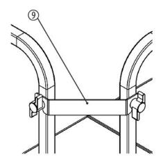
Finally, tighten the tommy screws of all mounting clamps firmly. Check the railings for firm fit.
