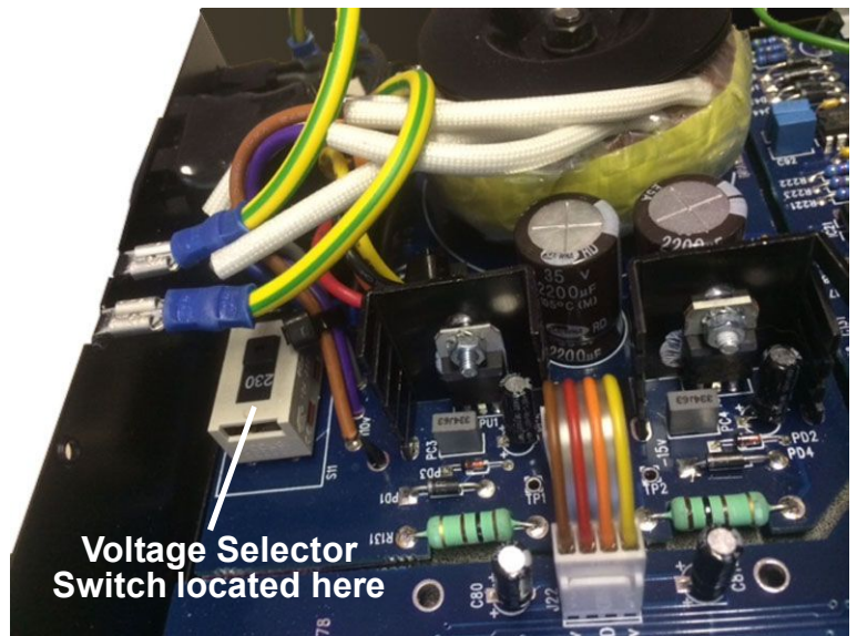
fig.2 The Voltage Selector Switch
