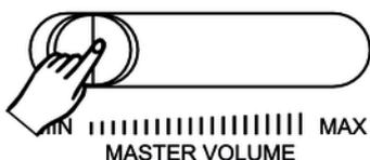
Adjust the volume control [MASTER VOLUME] for a pleasant volume for playback and practising. Slide the control to the right to increase the volume. Slide it to the left to decrease the volume.
