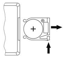
Press the lock of the battery holder to the centre of the housing and pull out the battery holder like a drawer. Insert the battery. The battery is correct if the positive pole points to the housing base of the remote control. Slide the battery holder back into the remote until it clicks into place.
