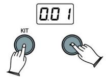
Press the [KIT] and [+] or [-] buttons simultaneously to adjust the pad volume. You also can select the individual pads by hitting them. Value range: '0' to '127'.
