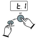
Press [KIT] and [REC/PLAY] simultaneously, then hit a pad for which you want to change the sound and use the [+] or [-] button to select the sound.
