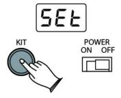
In this setup mode, you can adjust some global parameters according to your wishes and expectations. To enter the setup mode, switch off the drum module, then press and hold [KIT] while you switch it on again.
