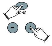
Press [SONG] and use the [+] or [-] buttons to set the velocity curve. There are four possible settings: 'NORM' (normal), 'DYNM' (dynamic) 'EASY' and 'FIXD' (fixed).
