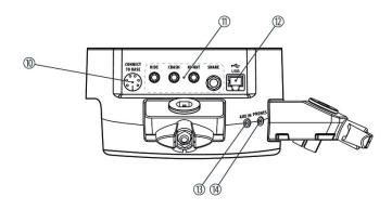
Connect the CONNECT TO BASE (10) terminal on the rear of the drum module with the CONNECT TO MODULE terminal on the rear of the bottom case using the included 6-pole cable in order to connect the bass-drum pedal and the hi-hat controller to the drum module.
