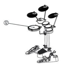
Place the snare drum (12) onto the shorter end of the L-piece snare drum support and tighten the wing nut on the holder clamp.
