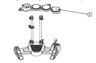
2. Insert the drum module with the three toms (4) into the stand tubes (2) and (3) and tighten the holder clamps on the wing nuts.
