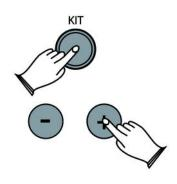
Press [KIT] and use the [+] or [-] buttons to set the trigger threshold. Value range: '001' to '050'.
