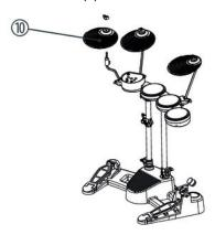
Place the hi-hat cymbal (10) onto the holder (7) as shown in the illustration and tighten the corresponding wing nut.
