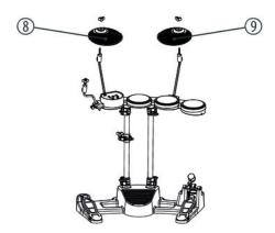
Place the two ride and crash cymbals (8) and (9) onto the cymbal holders (5) and (6) as shown in the illustration and tighten the corresponding wing nuts.
