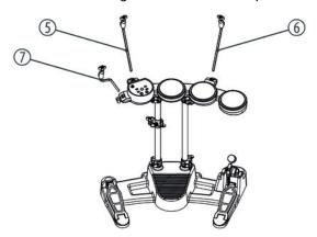
Insert the two longer cymbal holders (5) and (6) for the ride and crash cymbals and the shorter hi-hat holder (7) into the guides provided as shown in the illustration and tighten the wing nuts on the holder clamps.
