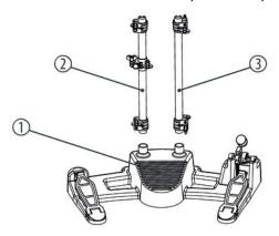
Put the bottom case with the bass-drum pedal and the hi-hat controller (1) on the floor. Insert the two stand tubes (2, with snare drum support) and (3) and tighten the wing nuts on the holder clamps.
