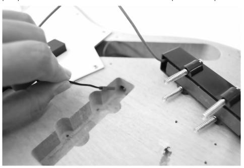
Fasten the pickup into the front recess using the screws provided.
