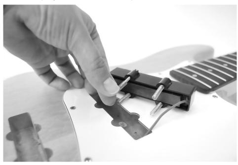
Screw the neck pickup into the recess for the pickguard using the supplied screws.
