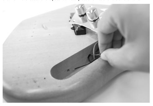
Pull the cable out of the hole far enough to ensure sufficient contact with the metallic surface when the bridge is installed. Earthing the strings reduces noise (humming).
