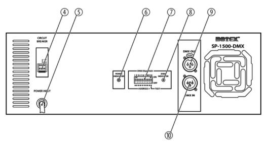
4 [CIRCUIT BREAKER] Line circuit breaker as automatic fuse. 5 [POWER INPUT] Mains cable for power supply. 6 [POWER INDICATOR] Indicates that the unit is connected to the power supply. 7 [DMX Dipswitch] DIP switches for setting the DMX address and operating mode. 8 [DMX INDICATOR] Indicates that a signal is present at the DMX input. 9 [DMX OUT] DMX output 10 [DMX IN] DMX input.
