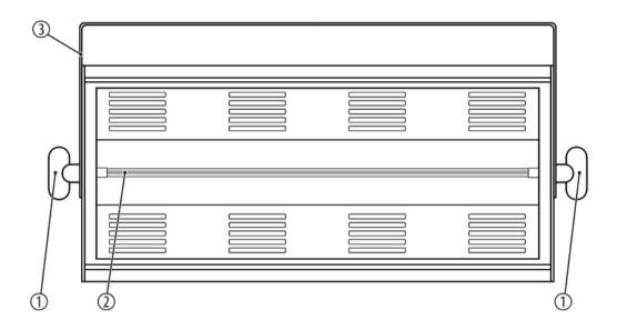
1 Locking screws for the mounting bracket 2 Illuminant 3 Mounting bracket
