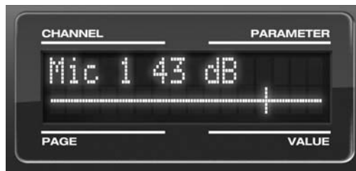
Figure 3-4: The LCD gives you feedback as you turn the TRIM knobs for the two mic/guitar inputs.
