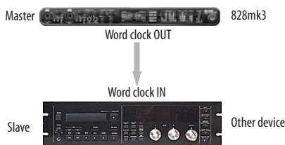
Figure 3-19: Slaving another digital audio device to the 828mk3 via word clock. For the 828mk3 clock source, choose any source besides word clock, as it is not advisable to chain word clock.
