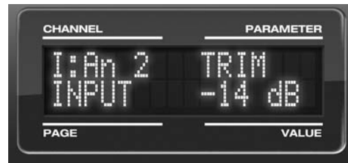
Figure 3-7: Setting the input trim for a TRS analog input pair.
