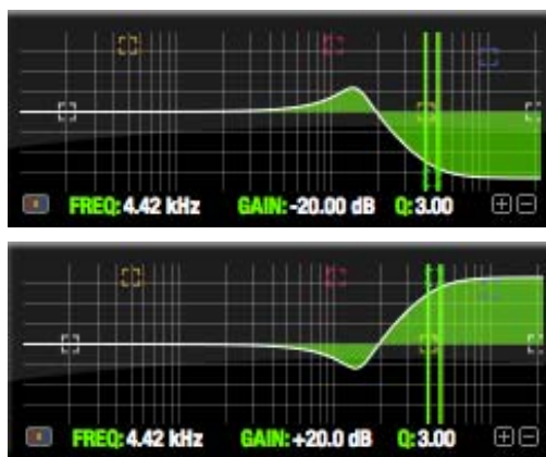
Figure 11-19: Overshoot when high shelf cut and boost is applied.
