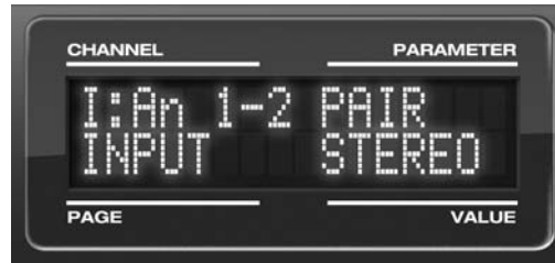
Figure 3-6: The settings for analog inputs 1 and 2 (as a pair).
