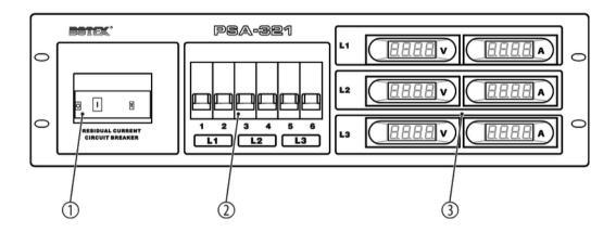
1 Residual current device (RCD). This protective device, also known as 'Fehlerstrom-Schutzschalter' or 'FI-Schalter' in German-speaking countries, is used for personal protection. As soon as it detects differential current / fault current, it automatically disconnects the device from the mains.
