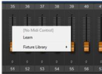
To associate a fader, dial or other DMXIS control with an external MIDI keyboard, right-click on the control and select *Learn*.
