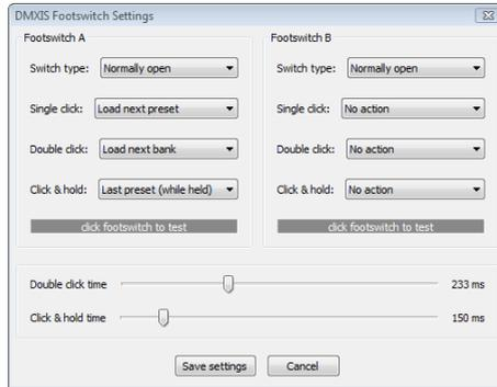
This window is accessed from the standalone DMXIS program (*Footswitch - Footswitch Settings* menu on OS X, *File - Footswitch Settings* menu on Windows). The settings applied here will also be used for the DMXIS plug-in.
