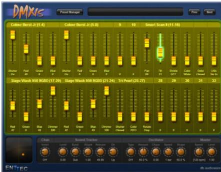
The 32 vertical faders are used to directly manipulate individual DMX channels. The channel number is shown above the fader, and the channel type & value is shown below.
