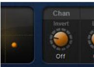
This control inverts the logical direction of all selected channels. For example, if you have a t-bar stand with four scanners, try inverting the *Pan* on scanners 3 & 4, and then move all four Pan controls at once. You'll see the scanner beams cross in the middle.
