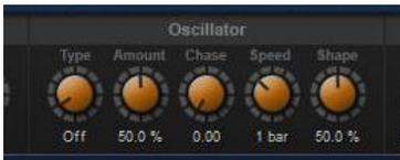
The oscillator lets you automatically sweep channel values up & down with a wide variety of “shapes”. *Although consisting of only 5 simple controls, the oscillator is the secret weapon in creating exciting moving visuals with DMXIS. This is the feature that*
