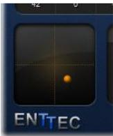
This control is normally disabled. It automatically enables when you select any channel in a light fixture with Pan/Tilt capabilities (for example, a scanner or moving head). Simply drag your mouse around to quickly position the fixture. You can <shift>drag for fine control.
