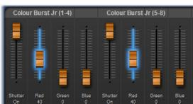
Double-clicking on any named channel (e.g. "Red") will automatically select ALL channels with that name on identical fixtures. This is a very handy short-cut when you need to make identical changes to a group of lights.
