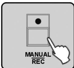
5. Press MANUAL/REC to store, LEDs on CUE, OVERRIDE, CENTRE, FIXTURE GROUP, PRESET, CHASE, BANK, BLACKOUT blink at the same time.
