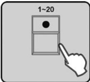
7. Press the number button 1-20 to select the scene to be inserted.
