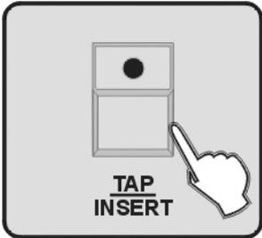
5. Press the button TAP/INSERT to insert a step following the present position.
