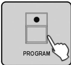
8. Press the button PROGRAM for three seconds to exit Program mode, the LED goes out indicating this selection.
