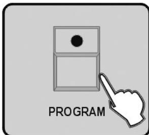
7. Press PROGRAM button for 3 seconds to exit Program mode, the LED goes out indicating this operation.
