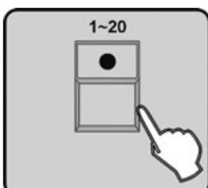
7. Press the number button 1-20 to store the edited scene which will cover the former scenes, all LEDs and the Segment Display will blink for three times briefly indicating this operation, then the LCD will show the bank and the scene number of the programmed scene.
