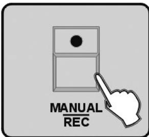
7. Press the button MANUAL/REC all LEDs blink for 3 times to indicate that you have successfully programmed a step.
