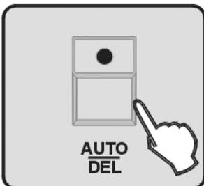
5. Press AUTO/DEL all LEDs blink for 3 times to indicate that you have successfully deleted the scene.
