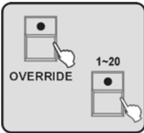
B. When CUE or CHASE or BANK running, press OVERRIDE button, then use 1-20 button to open the effect that be programmed.
