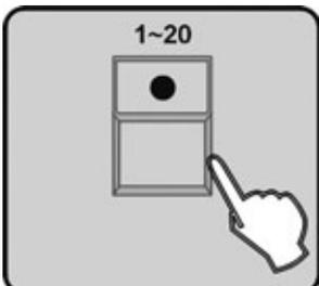
3. Press the number button 1-20 to select the chase number, the LEDs on BANK button will be all lit, the LCD will show the number and parameter of CHASE, BANK, SCENE, STEP, FADE, WAIT.
