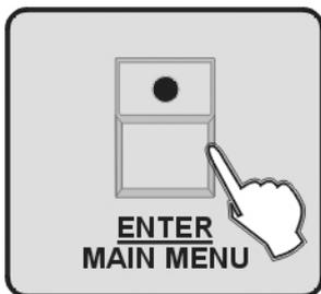
5. Press ENTER/MAIN MENU Button to enter, all the LEDs strobe for 3 times.
