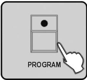
8. Press the button PROGRAM for three second, to exit Program mode, the LED goes out indicating this selection.
