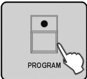
7. Press the button PROGRAM for three seconds to exit Program mode, the LED goes out indicating this selection
