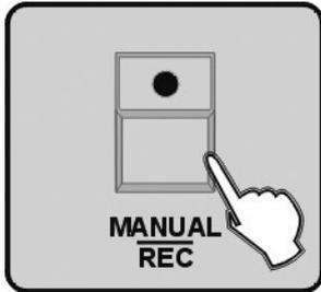
2. Press MANUAL/REC to into manual mode. The LED of MANUAL/REC will be on.
