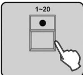
8. Press one of the number button 1-10 to store a COLOUR preset or press one of the number button 11-20 to store a GOBO preset, all LEDs blink for 3 times to indicate that you have successfully store a Preset.
