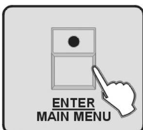
4. Press ENTER/MAIN MENU Button to set the address of the fixture, wait for 3 seconds, so the fixture can receive the signal of the controller and move all the motors to their "home" position.
