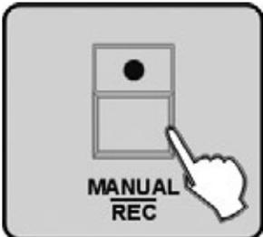
4. Once the scene is satisfactory, press MANUAL/REC button to program this scene into memory. At this moment, the LEDs on CUE, OVERRIDE, CENTRE, FIXTURE GROUP, PRESET, CHASE, BANK, BLACKOUT button blink at the same time.
