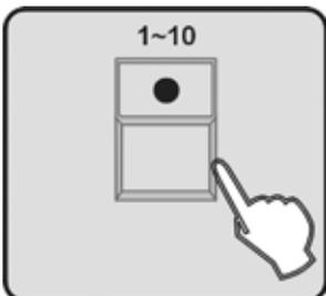
4. Use number Button 1-10 to input 6 digit old password (10 equal to number 0), if the password is wrong , it will hint to input continually.
