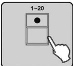
6. Press the number button 1-20 to select the Scene number going to be saved, all LEDs and the Segment Display will blink three times briefly indicating this operation, then the LCD will show the bank and the scene number of the programmed scene.
