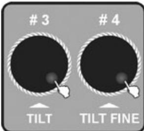
6. Use the Jog wheel #3, #4 to adjust the FADE TIME and WAIT TIME which are going to be added to the single Chase. If you do not make any adjustments, the system will remember the last FADE TIME or WAIT TIME.
