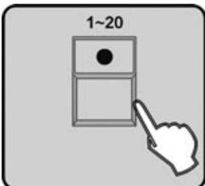
7. Press the number button 1-20 to select the to be stored Override number, all LEDs blink for 3 times to indicate that you have successfully preset an Override effect.
