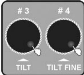
5. Use the Jog wheel #3 to adjust the FADE TIME of present chase, the Jog wheel #4 to adjust the WAIT TIME of the present chase. If you do not make any adjustments, the system will remember the last FADE TIME or WAIT TIME.
