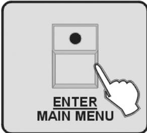
6. Press ENTER/MAIN MENU Button to enter, all the LEDs will blink for 3 times.
