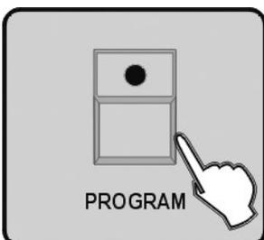
10. Press the button PROGRAM for 3 seconds to exit Program mode, the LED goes out indicating this operation.
