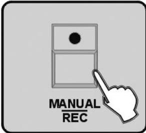
7. Press the button MANUAL/REC, all LEDs blink for 3 times, all the programmed scenes in the Bank will join the Chase.
