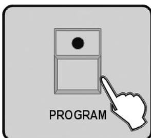
7. If you don't intend to continue your programming, press and hold down the PROGRAM button for three seconds to exit Program mode, the LED goes out indicating this selection
