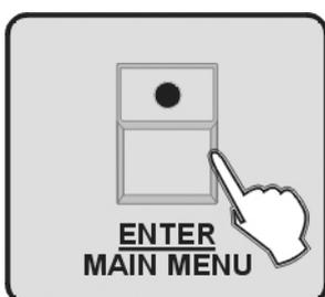
8. Press ENTER/MAIN MENU button, all LEDs blink for 3 times to indicate that you have successfully edited a FIXTURE PROFILE.
