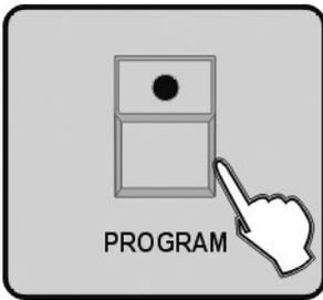
8. Press PROGRAM button 3 seconds to exit Program mode, the LED goes out indicating this operation.
