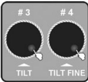
5. Use the Jog wheel #3, #4 to adjust the FADE TIME and WAIT TIME which are going to be added to the single Chase. If you do not make any adjustments, the system will remember the last FADE TIME or WAIT TIME.
