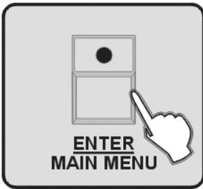
3. The LCD hint to input 6 digit memory protect password. Input the exact password, and Press ENTER/MAIN MENU Button to delete the memory information. You have to input the password again when it's wrong.
