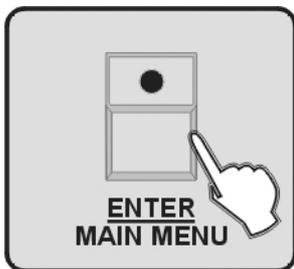
4. Press ENTER/MAIN MENU Button to enter, all the LEDs will blink for 3 times, then back to the last menu.
