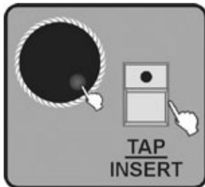
4. Use Jog wheel #3 or #4 to adjust current FADE TIME or WAIT TIME, or use TAP/INSERT Button to adjust the speed of the scene.
