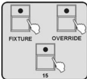
Format the program of the controller, then download the last software and copy to CF:\SUP2420\APP2420.SUP, inset the CF card to the seat, press FIXTURE and OVERRIDE and number button 15 then Power on afresh until the information show on the LCD display, the controller will test if the CF card stick well and then update the new software, it will cost about 20 seconds, please don't move the CF card or cut the power in order to avoid update frustrated and damage the CF card.
