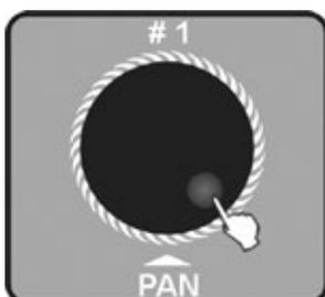
3. Use Jog wheel #1 to select the bank you need, then the scene in the bank will run with music. When it is running the scene with Movements in sound activation mode, it will process repeatedly as per the built in movement Loop time then enter next step.
