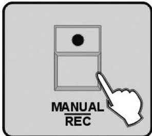
4. Once the effect is adjusted, press MANUAL/REC button to store, at this moment, all LEDs on CUE, OVERRIDE, CENTRE, FIXTURE GROUP, PRESET, CHASE, BANK, BLACKOUT blink at the same time.
