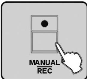
4. Press MANUAL/REC button, at this moment, all LEDs on CUE, OVERRIDE, CENTRE, FIXTURE GROUP, PRESET, CHASE, BANK, BLACKOUT blink at the same time.
