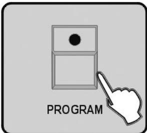
5. Press PROGRAM button for 3 seconds to exit Program mode, the LED goes out indicating this operation.
