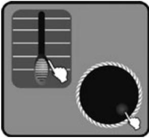
6. Move FADERS 1-24 and use Jog wheel #3, #4 to change the centre position of PAN, TILT where you desired. (The codes of the channel feature of ARRT CODE are "P", "PF", "T", "TF" in the fixtures bank) for the convenience to check other channels, there would be some output of the channels, but the channel output will not be stored in the centre.
