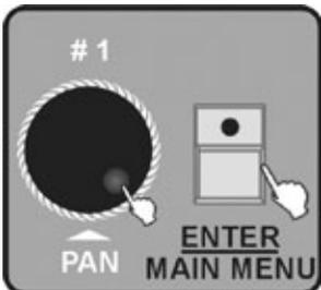
3. Use Jog wheel #1 to read the program file 01. Load program file or profile file 02. Load a fixture profile. Press ENTER/MAIN MENU button to enter.
