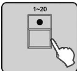
6. Then press the number button 1-20, the scene will be deleted, all LEDs and the Segment Display will blink for three times briefly indicating this operation, then the LCD will show the bank and the scene number of the deleted scene.
