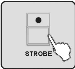
3. Control: Press STROBE button then the controller will control the DMX strobe light with the value of the DMX be set, and the light strobe in the speed that be set to the simulate strobe light.
