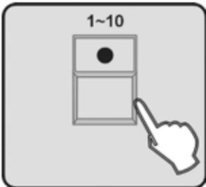
4. Press the button 1-10 to select one MOVEMENT in ten, the selected FIXTURE will run the MOVEMENT.
