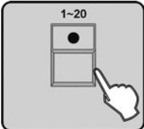
9. Press the number button 1-20 to select the location to store the Centre, all LEDs blink for 3 times to indicate that you have successfully edited a Centre position.
