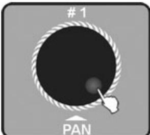
4. The list of the program/profile files will show on the LCD, turn jog wheel #1 to select the file name. The amount of the files consider to the amount of the program or profile files which you saved under the directory of DIR2420 in the CF card.
