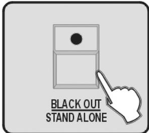
5. Press BLACK OUT/STAND ALONE button, all LEDs blink for 3 times to indicate that you have successfully stored a Black Scene.
