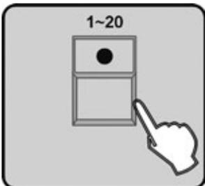
6. Press the number button 1-20, then copy the Scene to the right position. All LEDs and the Segment Display will blink for three times briefly indicating this operation, then the LCD will show the bank and the scene number of the programmed scene.
