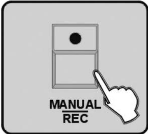
5. Press MANUAL/REC Button, at this moment, all LEDs on CUE, OVERRIDE, CENTRE, FIXTURE GROUP, PRESET, CHASE, BANK, BLACKOUT blink at the same time.
