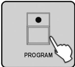
6. Press PROGRAM button for 3 seconds to exit Program mode, the LED goes out indicating this operation.
