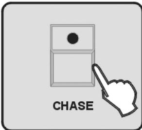
9. Finally press the button CHASE to store the chase then exit the programming state.
