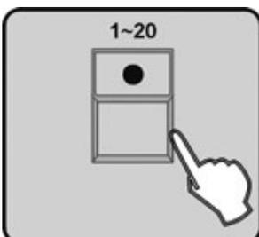
6. Press the number button 1-20 to select the number of the fixture group for store, all LEDs blink for 3 times
