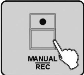
4. Press MANUAL/REC to store, LEDs on CUE, OVERRIDE, CENTRE, FIXTURE GROUP, PRESET, CHASE, BANK, BLACKOUT blink at the same time.
