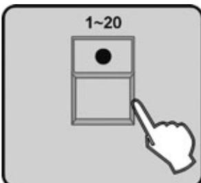
3. Press the number button 1-20 to select the Chase number, LEDs on the BANK button will be all lit, the LCD will show the number and parameter of the CHASE, BANK, SCENE, STEP, FADE, WAIT.
