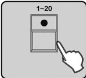
3. Press the number button 1-20 to select one or more fixtures to make the fixture group.
