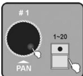
3. Press the number button 1-20, to select the to be edited CUE number, at this moment, all LEDs on CHASE are lit and all LEDs on the number button which have saved CHASE will blink. Turn jog wheel #1 should change the page number.
