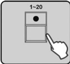
4. Press the number button 1-20 to select the chase to be deleted, all LEDs blink for 3 times to indicate that you have successfully delete the chase.
