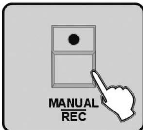
7. Press MANUAL/REC button, at this moment, all LEDs on CUE, OVERRIDE, CENTRE, FIXTURE GROUP, PRESET, CHASE, BANK, BLACKOUT blink at the same time.
