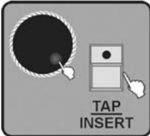
4. Setting to CHASE RUN BY INSIDE TIME, then it will run as the FADE TIME or FADE TIME of the step that you set when store the chase. Setting to CHASE RUN BY OUTSIDE TIME, then it will run as the FADE TIME or FADE TIME you set last time, you can also adjust by turn the joy wheel #3 or #4, or use TAP/INSERT Button to adjust the speed.
