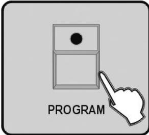
11. Press PROGRAM button for 3 seconds to exit Program mode, the LED goes out indicating this operation.
