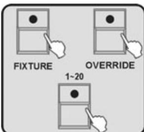
A. When CUE or CHASE or BANK running, press OVERRIDE button, Then press FIXTURE button, and use number button 1-20 to choose light, so you can push the handspike to change the effect.
