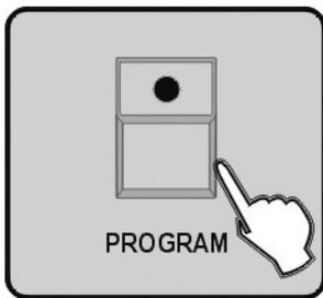
11. If you don't intend to continue your programming, press and hold down the PROGRAM button for three seconds to exit Program mode, the LED goes out indicating this selection.
