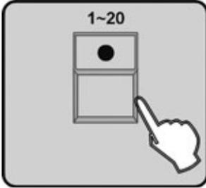
7. Press the number button 1-20 to select the location to store the Centre all LEDs blink for 3 times to indicate that you have successfully stored a Centre position.
