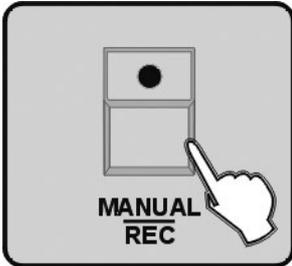
5. Press the button MANUAL/REC at this moment all LEDs on buttons CUE, OVERRIDE, CENTRE, FIXTURE GROUP, PRESET, CHASE, BANK, BLACKOUT blink at the same time.
