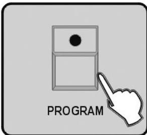
10. Press the button PROGRAM for three seconds to exit Program mode, the LED goes out indicating this selection.
