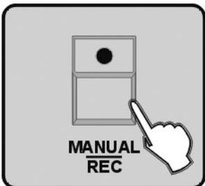
8. Press MANUAL/REC button , at this moment, all LEDs on CUE, OVERRIDE, CENTRE, FIXTURE GROUP, PRESET, CHASE, BANK, BLACKOUT blink at the same time.
