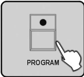
6. Press the button PROGRAM for 3 seconds to exit Program mode, the LED goes out indicating this operation.
