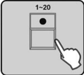
6. Press number Button 1-20, all the LEDs will blink for 3 times, the address of the corresponding fixture will show on the LCD display, it means the fixture's amount of the channel is as same as the corresponding number button's.
