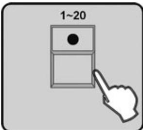
4. Then press the number button 1-20, all LEDs blink for 3 times to indicate that you have successfully deleted a CUE.
