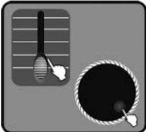
3. Slide Faders 1-24 or use the CENTRE or PRESET or SCENE have saved to change the output of each channel. You can also use the jog wheel #1 & #2 to control the PAN, PAN FINE or use the jog wheel #3 #4 to control TILT, TILT FINE.
