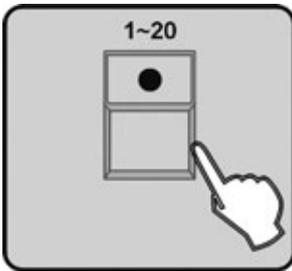
8. Press the number button 1-20 to select the fixture group number you selected in step 2, all LEDs blink for 3 times
