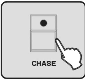
11. Press the button CHASE to store the chase and exit the chase programming state.
