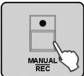
9. Press the button MANUAL/REC all LEDs blink for 3 times to indicate that you have successfully inserted a step into a chase.
