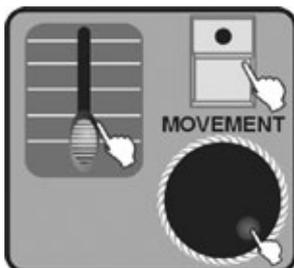
4. Move Faders 1-24 or use the CENTRE, PRESET, SCENE have saved to change the output of each channel, you can also use the Jog wheel #1, #2 to adjust PAN, PAN FINE, or use Jog wheel #3, #4 to adjust TILT, TILT FINE or press MOVEMENT to add MOVEMENT function.
