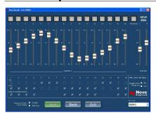
The 8804 provides balanced Direct Outputs from each of the 16 channels. These can be used for recording or as sends to effects units and processors.
