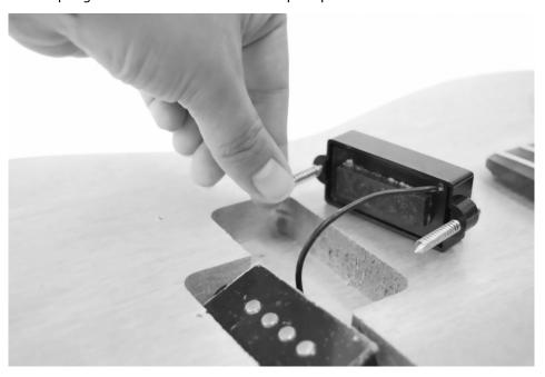
Screw the pickups into the recess in the guitar body using the supplied screws.
