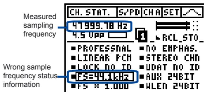
Fig 5-06, Channel status consistency check
