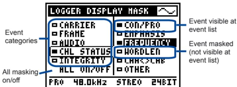
Fig 5-24, Logger display mask
