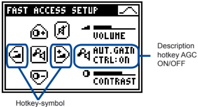
*Fig 2-08, Automatic gain control*
