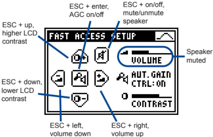
*Fig 4-09, Fast access setup screen*
