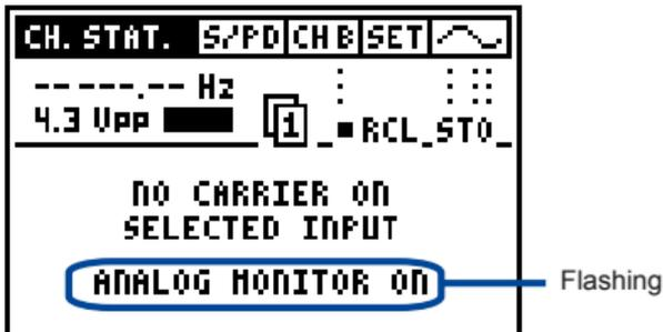
Fig 2-07, Analog monitoring
