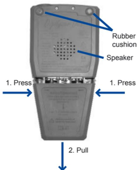
*Fig 2-10, Open battery compartment*
