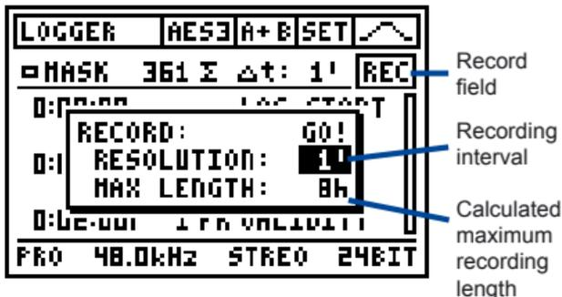
Fig 5-21, Recording setup window
