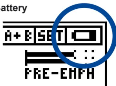
Fig 4-06, Low battery indicator
