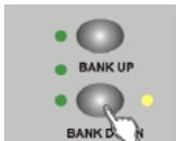
2. Use the Bank Up/Down button to select the DMX channel 01-16 to assign to MIDI channel.
