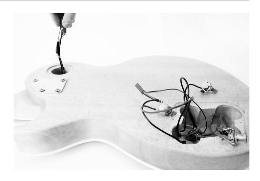
Then put the potentiometers into the opening in the back as shown in the following picture.
