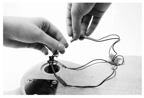
Place the plastic cover and a washer in place and fasten the switch with the nut provided. The neck pickup is generally activated with the switch in the upper position, and the bridge pickup in the lower position. This configuration can be changed at any time simply by swapping the two connectors.
