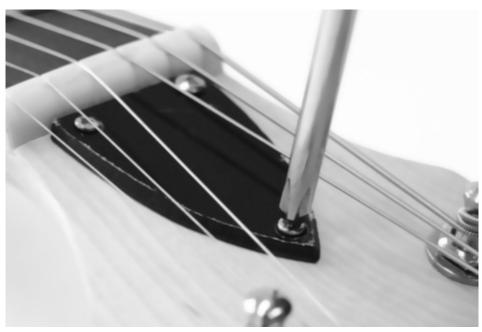
Screw the cover for the truss bar onto the header headstock.
