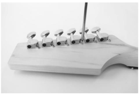
Turn the neck and fasten all the machine heads finger-tight to the front of the headstock with the washers and nuts provided.
