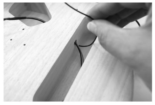
Run the cable for earthing the strings (stripped, without connectors) through the channel in the recess for the potentiometer plate and into the recess for the bridge pickup.
