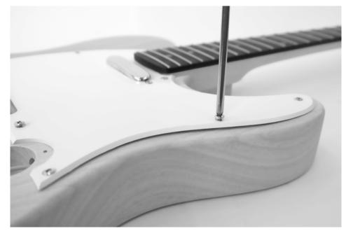
Position the pickguard over the front of the body so that the neck pickup is seated in the correct recess. Screw the pickguard onto the body using the screws provided.
