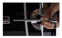
Hand-tighten all eight screws. When doing this, tighten the screws in the diagonally opposite sequence. You only need to tighten the screws slightly, we will be tuning the drums later on.
