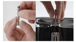
You hand-tighten the tension rods in the diagonally opposite sequence. Now assemble the second hanging tom in exactly the same way as the first one. Like the bass drum, we will be tuning the tom later on.
