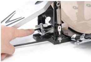
Now you can push the assembled bass drum pedal onto the clamping ring and fix it with the claw. Use some gaffa tape to protect the hoop from scratching.
