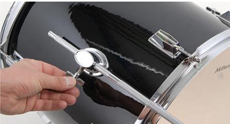
You can now attach the legs. When doing this, turn the feet outwards to ensure as much stability as possible. Fix the two legs at the back in about the middle. First lightly fix the leg facing the drummer by hand and then fasten it properly when it is standing. Hold the shell with one hand while screwing it with the other one.
