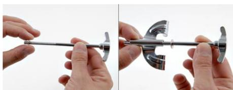
Proceed as follows: Put the washer on the screw and then the claw hook. We need six wing screws and two square-head ones. The two square-head screws are on the bottom, i.e. opposite the tom holder so that there is enough free space on the ground later on.
