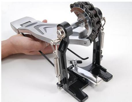
In fact, there are two round iron rods that are spring-urged to press outwards. You can press them together with one hand and push them into the cutouts on the frame of the bass drum pedal. If the bass drum pedal has a floor plate, you don't need to carry out this step.
