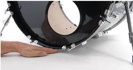
We adjust the length of the spurs such that there is a gap of the width of one finger between the floor and the lower edge of the hoops; when doing this, the drum shell should not lean forwards or towards the player. To retain the settings of the spurs, the bass drum spurs for height adjustment are fitted with memory clips (that remain in position at dismantling too.) You must use the drum key to fix the screws.
