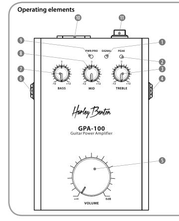
PEAK This LED lights up on excessive input signal **TREBLE** Treble control **INPUT** Input of the device VOLUME Volume control **OUTPUT** Output of the device BASS Bass control 8 MID Mid control 9 PWR/PRO Power ON indicator / Indicator for activated protection circuit
