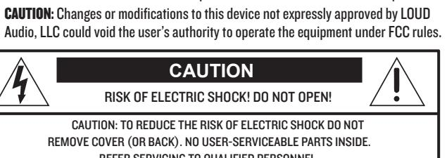
The lightning flash with arrowhead symbol within an equilateral triangle is intended to alert the user to the presence of uninsulated "dangerous voltage" within the product's enclosure, that may be of significant magnitude to constitute a risk of electric shock to persons.
