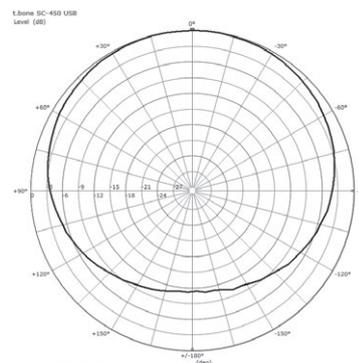
Polardiagramm @ 1 kHz
